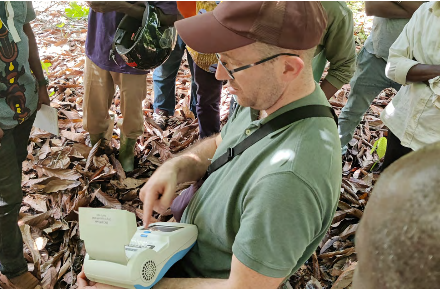
The DNAFoil CSSVD test is easy to perform and allows anyone out in the fields to quickly test cocoa trees, using their leaves as samples.
